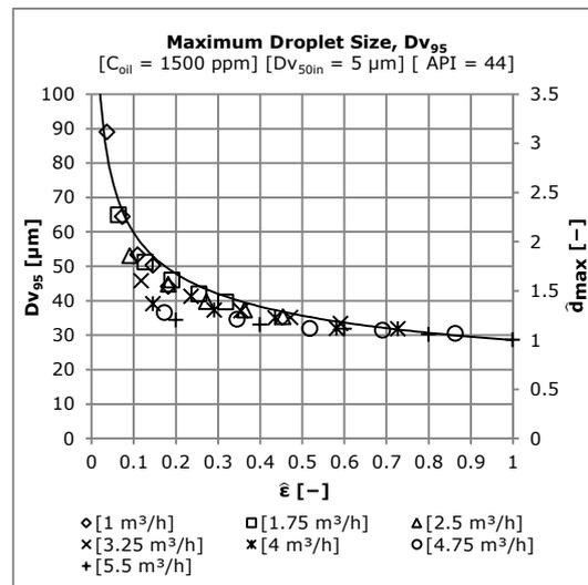
Figure 5 – Measured maximum droplet size ( $Dv_{95}$ ) and estimated normalised maximum droplet size ( $\hat{d}_{max}$ ) as a function of the normalised turbulent energy dissipation rate ( $\hat{\epsilon}$ ) for various points of operation.
