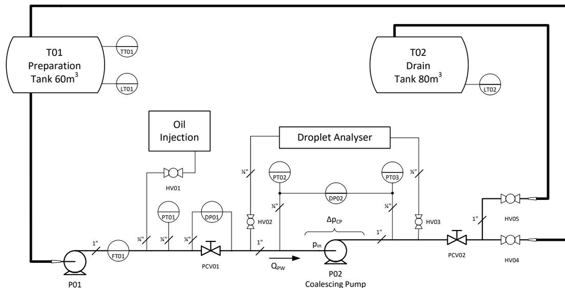
Figure 1 – Schematics of the Coalescing Pump Test Rig.
