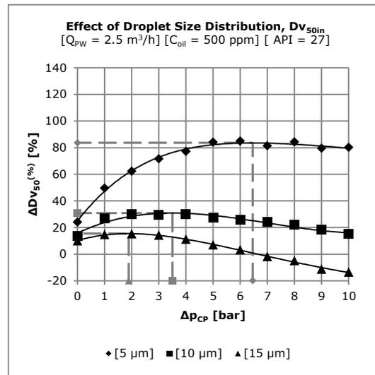
Figure 8 – Percentage change of  $Dv_{50}$  ( $\Delta Dv_{50}^{(\%)}$ ) with respect to the pumping pressure ( $\Delta p_{CP}$ ) for different inlet droplet size distributions ( $Dv_{50in}$ ).
