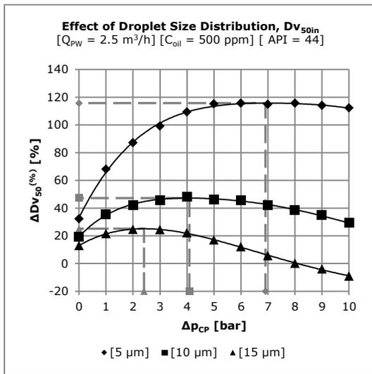
Figure 7 – Percentage change of  $Dv_{50}$  ( $\Delta Dv_{50}^{(\%)}$ ) with respect to the pumping pressure ( $\Delta p_{CP}$ ) for different inlet droplet size distributions ( $Dv_{50in}$ ).
