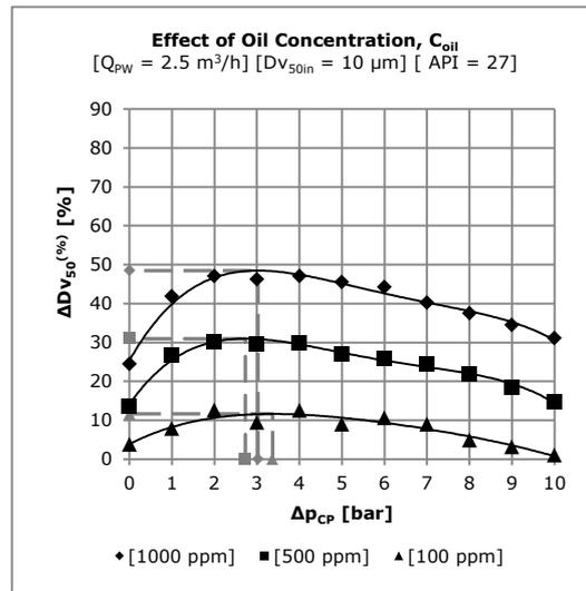
Figure 10 – Percentage change of  $Dv_{50}$  ( $\Delta Dv_{50}^{(\%)}$ ) with respect to the pumping pressure ( $\Delta p_{CP}$ ) for different oil concentrations ( $C_{oil}$ ).
