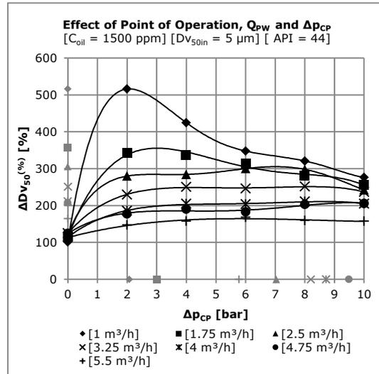
Figure 6 – Percentage change of  $Dv_{50}$  ( $\Delta Dv_{50}^{(\%)}$ ) with respect to the pumping pressure ( $\Delta p_{CP}$ ) for different flow rates ( $Q_{PW}$ ).  $Dv_{50in} = 5 \mu\text{m}$ ,  $Q_{PW} \in \{1, 1.75, 2.5, 3.25, 4, 4.75, 5.5\} \text{ m}^3/\text{h}$ ,  $C_{oil} = 1500 \text{ ppm}$  and  $\text{API} = 44$ .
