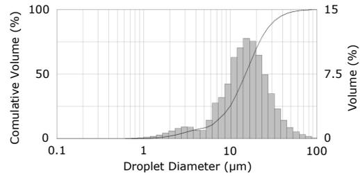
Figure 4 – Typical inlet droplet size distribution with  $Dv_{50} = 15 \mu\text{m}$ .
