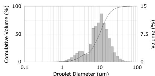
Figure 3 – Typical inlet droplet size distribution with  $DV_{50} = 10 \text{ }\mu\text{m}$ .
