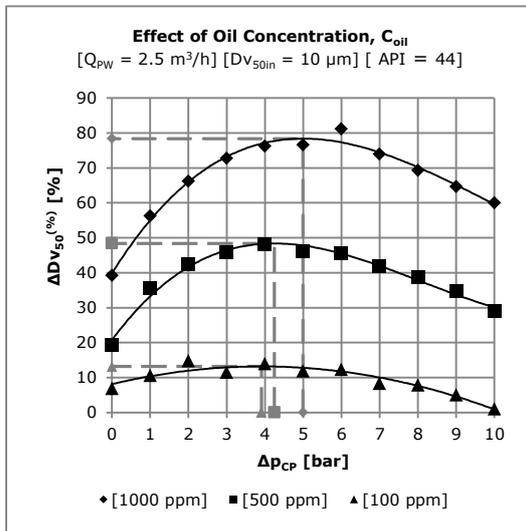
Figure 9 – Percentage change of  $Dv_{50}$  ( $\Delta Dv_{50}^{(\%)}$ ) with respect to the pumping pressure ( $\Delta p_{CP}$ ) for different oil concentrations ( $C_{oil}$ ).
