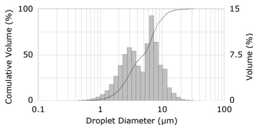
Figure 2 – Typical inlet droplet size distribution with  $DV_{50} = 5 \text{ }\mu\text{m}$ .
